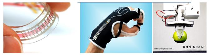
(Left) detail of a stretchable pump and (center) a pump and fluidic muscles mounted on a glove for muscle support and thermal regulation, *Nature 2019.* (Right) Omnigrasp soft gripper lifting fruit using silicone fingers and electro-adhesion.
