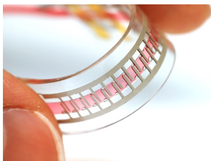
(Left) detail of a stretchable pump and (center) a pump and fluidic muscles mounted on a glove for muscle support and thermal regulation, Nature 2019. (Right) Omnigrasp soft gripper lifting fruit using silicone fingers and electro-adhesion.
