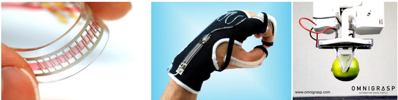
(Left) detail of a stretchable pump and (center) a pump and fluidic muscles mounted on a glove for muscle support and thermal regulation, Nature 2019. (Right) Omnigrasp soft gripper lifting fruit using silicone fingers and electro-adhesion.
